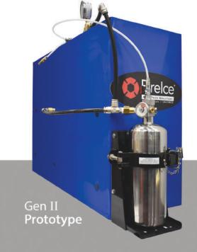
The Lithium Battery Active Suppression Kit automatically detects elevated temperatures to cool, suppress, and prevent battery runaway. It's modular design keeps potential incidents self-contained by dispensing cooling FireIce® ST gel only to compartments where temperatures reach 165° F (customizable for higher or lower temperatures). FireIce® ST cools and suppresses only where needed and prevents the spread of runaway to adjacent battery cells.
